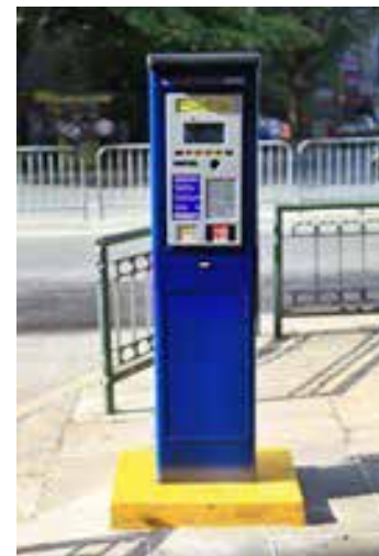
Figure 5: Solar Powered Parking Meters
